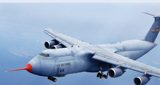
The C-5M transport with the 100510-08 air data boom leading the way.
