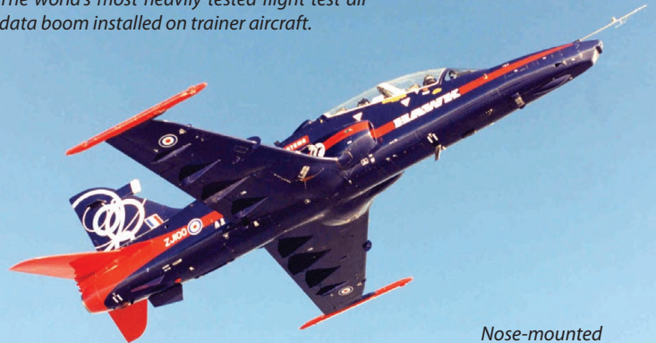
Nose-mounted 100700-051 air data boom (air)
