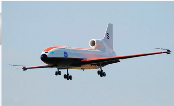
NASA Langley S2 aircraft (1/24 scale L-1011) with 101100 subminiature air data booms on each wingtip.
